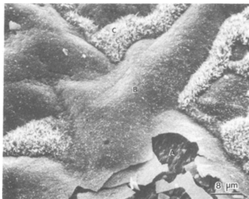
Figure 1 Scanning electron micrograph showing \alpha\text{-Fe}_2\text{O}_3 de-cohesion and cracking, A, blistering, B, and blade growth, C, during the early period of oxidation (sample oxidized for 5 min at 600^\circ\text{C} ).
